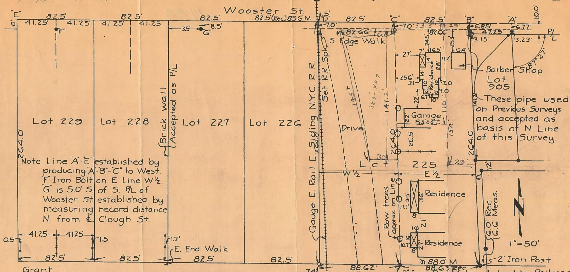
Note Line "A"-E established by producing "A"-B-C to West. "F" Iron Bolt on E Line W 1/2. "G" is 5.0' S. of S. P/L of Wooster St. established by measuring record distance N. from Clough St.
