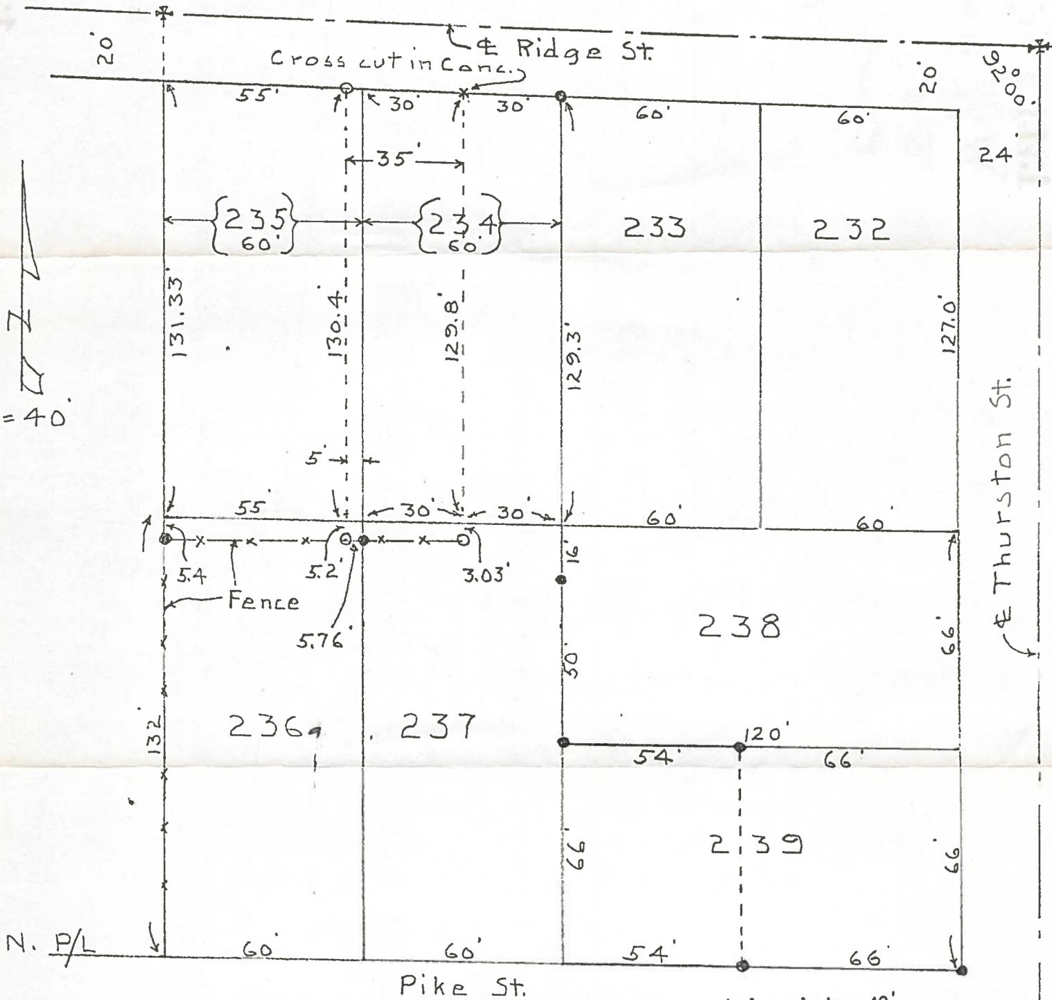
In making this survey the width of Ridge St. was accepted as being 40' as no width is shown on the Original Plat ( Vol.1, Page 75 of Wood Co. Plats). The south line of the parcel surveyed is north of the occupational line. Pipe were set on the occupational line. Nothing of a structural nature should be erected in the space between our line and the occupational line.
