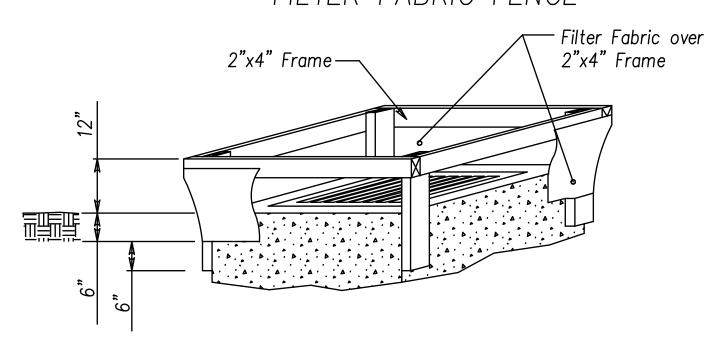
MATERIALS: Filter Fabric shall meet the requirements of CMS 712.09, Type C. The framing wood shall be construction grade 2"x4" lumber.
