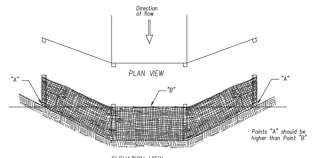
ELEVATION VIEW PLACEMENT AND CONSTRUCTION OF DITCH CHECK FILTER FABRIC FENCE
