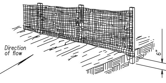
Place fabric and support stakes and extend fabric into the trench.
