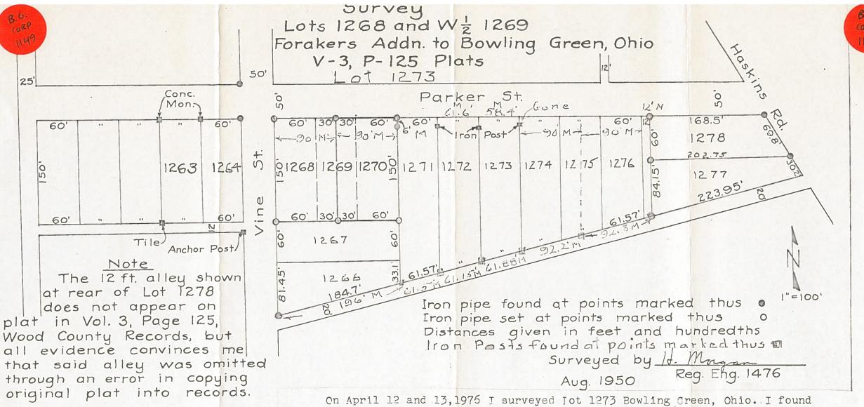
On April 12 and 13,1976 I surveyed Iot 1273 Bowling Green, Ohio. I found the iron posts set on the southerly side of Lots 1276 to 1271 to be in error, the alley width was evidently omitted in figuring the width of Lot 1276 as a 11.3 foot surplus appears on Lot 1266, Post at north west corner of Lot 1273 encroaches 1.6 feet on the said Lot. Measurements taken on this Survey are marked "M." I advise using the area posts as they have been in place for over 26 years.
